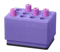
Thermoconductive Tube Rack for 12 x 13mm or 16mm Blood Tubes, with Insulative Exterior are precision-engineered sample modules manufactured from a novel thermo-conductive alloy material, designed to evenly distribute temperature across all wells providing uniform and consistent temperature to all samples (+/-0.1°C)
