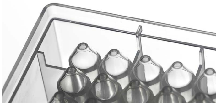
Fig. 4 Special shape of the stacking ribs - the plate sits much lower on the magnetic separator than standard round well plates thus facilitating the speed and efficiency of the separation process.
